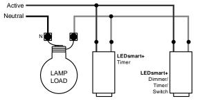
Two-way control using an LEDsmart+ timer and an additional LEDsmart+ switch, dimmer or timer. Note these devices are simply wired in parallel.
